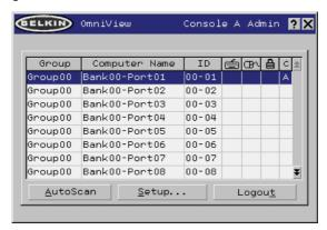
The Main page displays information regarding the current connected severs. At a glance, the user can view the server's group, computer name, port locations, connection status, and security mode. The Main page could also be used to navigate through the connected server.
